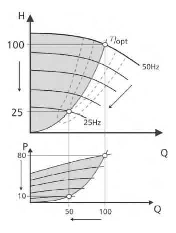
• a lowering of the flow acc. to the linear function
