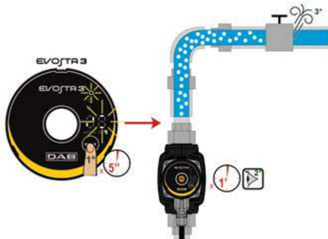
Figure 8: Automatic venting of the pump
