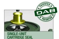
A single-unit cartridge seal is a great advantage for maintenance of the pump as allows the removal and insertion of the seals in less time, having a total guarantee to carry out properly. It's an **exclusive patent DAB**: a double mechanical seal Sic-Sic with opposite faces, independent from the rotation direction of shaft, with Viton elastomers and leap seal.
