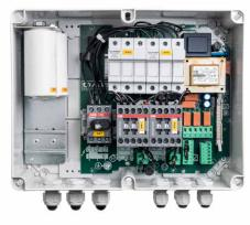
**e.box plus** is an electronic control panel for the protection and automatic operation of one or two submersible pumps or pressurizing both single-phase and three-phase, installed in domestic, civil and industrial environments. Thanks to the possibility of adjusting the current, **e.box** is compatible with all models of pumps with a current between 1 and 12A with power up to 5.5Kw as reported by the products compatibility chart.
