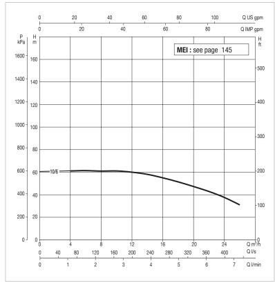
The performance curves are based on kinematic viscosity values  $= 1 \text{ mm}^2/\text{s}$  and density equal to  $1000 \text{ kg/m}^3$ . Curve tolerance according to ISO 9906. Overall performance taking into account TWO pumps working at the same time.
