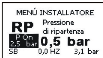
Figure 18: Setting the restart pressure
