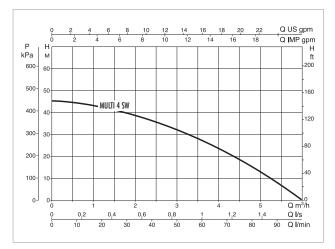
The performance curves are based on kinematic viscosity values =  $1~\text{mm}^2/\text{s}$  and density equal to  $1000~\text{kg/m}^3$ . Curve tolerance according to ISO 9906.
