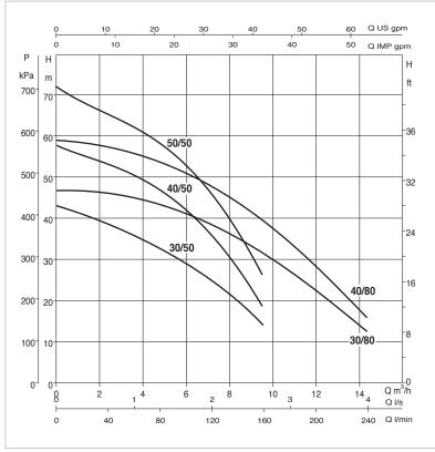
The performance curves are based on kinematic viscosity values = 1  $\text{mm}^2/\text{s}$  and density equivalent to 1000  $\text{kg/m}^3$  Curve tolerance according to ISO 9906.
