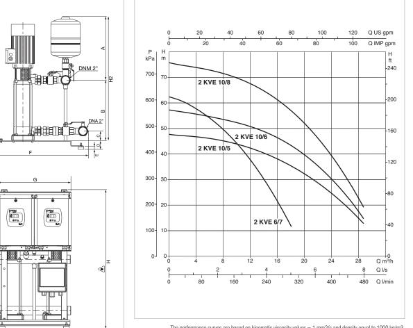
The performance curves are based on kinematic viscosity values = 1 mm2/s and density equal to 1000 kg/m3. Curve tolerance according to ISO 9906. Overall performance taking into account TWO pumps working at the same time.
